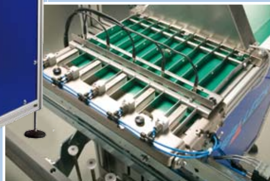
Special Teflon insert to guide the blanks carefully on top of each other
