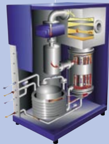
Evaporator for total water recycling
